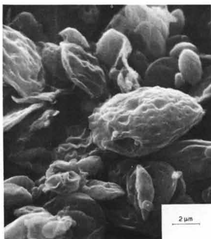
Figure 8 Biaxially oriented rubber particles due to vacuum forming
